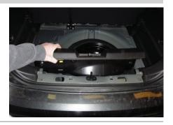
Use the panel trim removal tool to loosen the side wall panels and carefully pull the panel out. Locate the vehicle taillight wiring connectors. The connectors will be similar to those on your new RV harness product. Separate the connectors from the taillight housing taking care not to damage the locking tabs.
